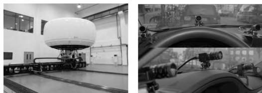
图5 同济大学 8 自由度驾驶模拟器和 Smart Eye® 眼动仪 Fig. 5 Tongji 8 DOF advanced driving simulator and Smart Eye® eye tracker
